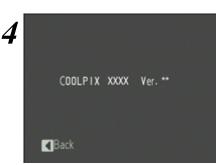
The current firmware version will be displayed. Confirm that the firmware version is the correct version for this update.
